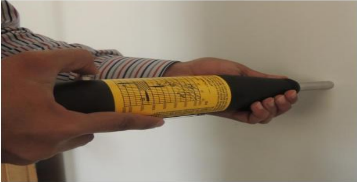
Figure – 2: Rebound hammer in use
