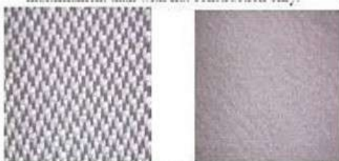
Fig 1. Woven Geotextile Fig 2. Non-woven Geotextile
