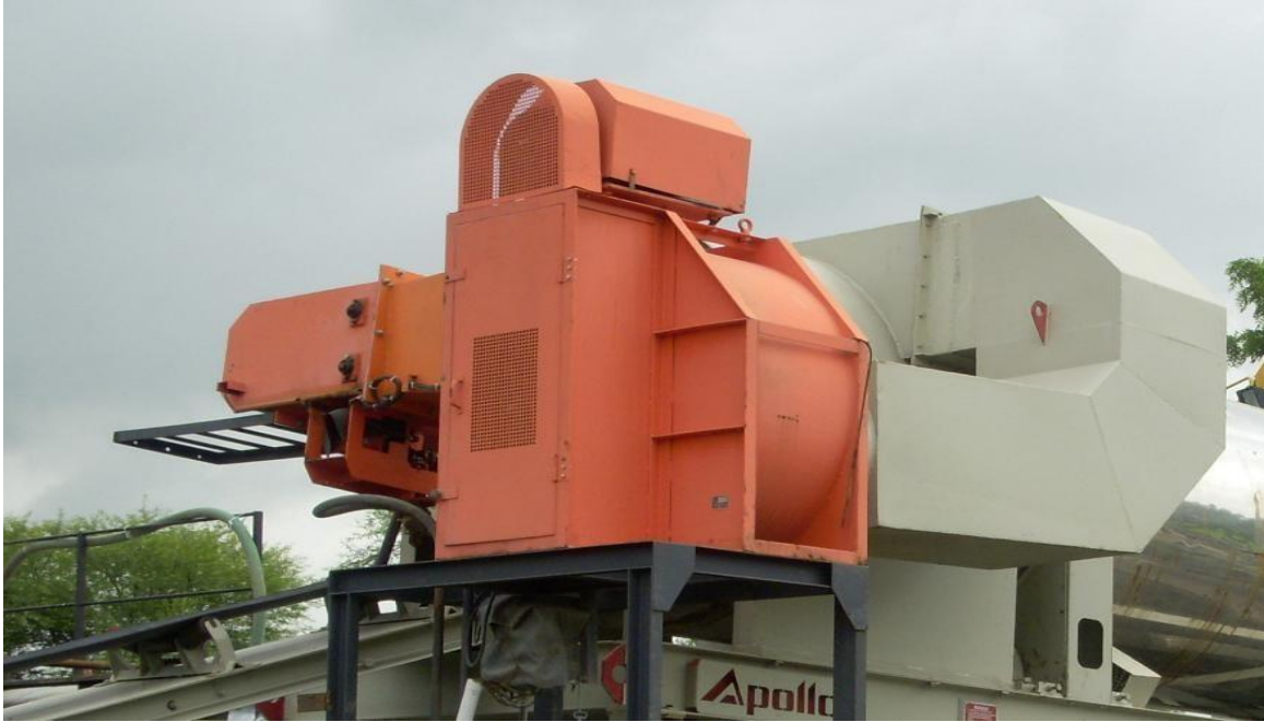
Fig. Aggregate Dryer
