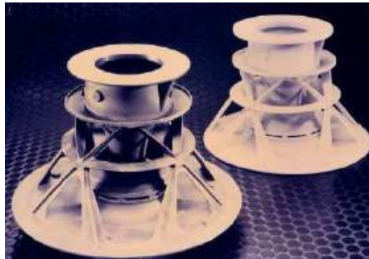
Cast metal (left) and RP pattern for sand casting (Courtesy of Helysis Inc.)
