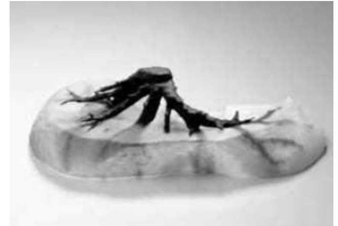
Objet Connex process showing vascularity inside a human organ
