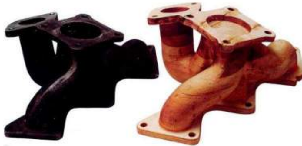
Cast metal (left) and RP pattern for sand casting (Courtesy of Helysis Inc.)
