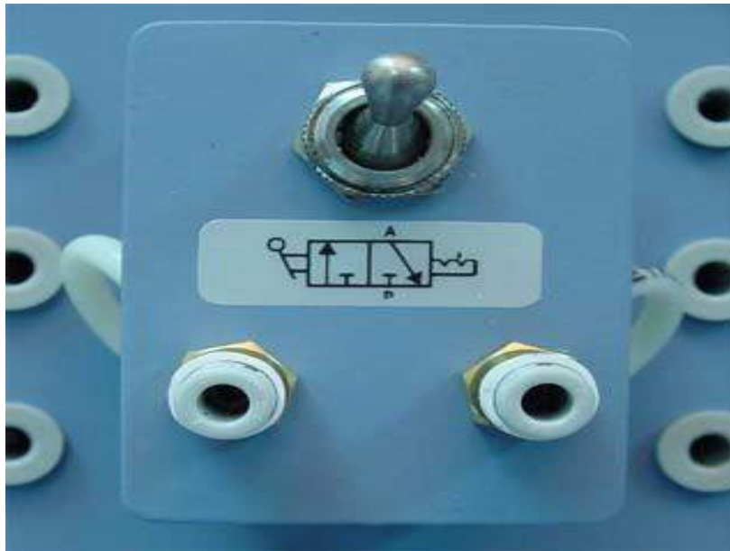
Fig. 10 (a) 3/2 directional control valve (b) Cross section
