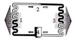
A diagram of a simple heat pump's vapor compression refrigeration cycle: 1) condenser, 2) expansion valve, 3) evaporator, 4) compressor.
