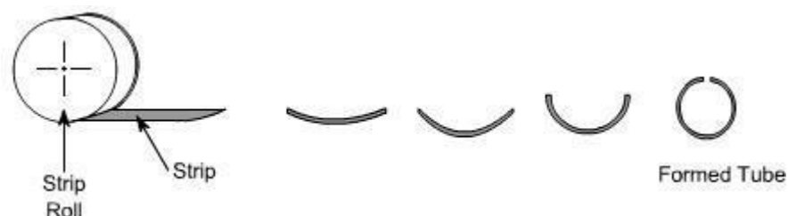
Fig 11.10: Forming of Tube from Strip
