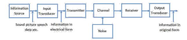
The essential components of a communication system are information source, input transducer, transmitter, communication channel, receiver and destination.
