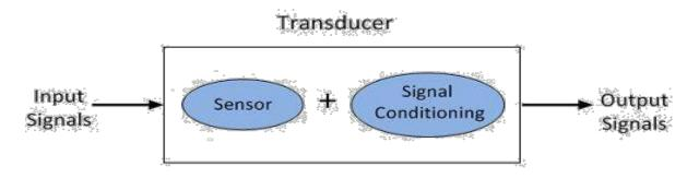
The transducer has three major components; they are the input device, signal conditioning or processing device and an output device.
