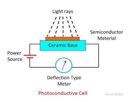
When the beam of light falls on the semiconductor material, their conductivity increases and the material works like a closed switch. The current starts flowing into the material and deflects the pointer of the meter.
