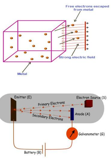
velocity striking electrons, transferred to the free electrons on the metal surface. Thus the free electrons may get sufficient kinetic energy to overcome the surface barrier and knocked out from the surface & start electron emission.
