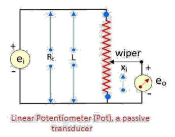
Consider the L is the length of the potentiometer.  $R_i$  is their total internal resistance and  $x_i$  is their input displacement. The output voltage is calculated by the formula shown below.
