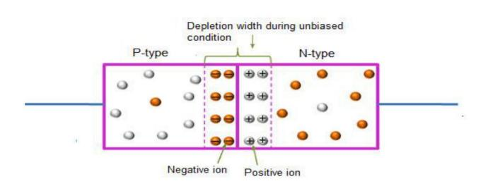
This pn junction does not allow flow of current. To make it suitable for electronics circuits we need to biasing (applying external voltage) pn-diode. There are two ways of biasing pn-diode (i) Forward biasing
