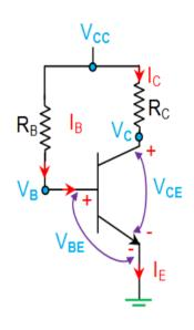
Transistor biasing was done with the aid of a battery  $V_{BB}$  which was separate from the battery  $V_{CC}$  used in the output circuit. However, in the interest of simplicity and economy, it is desirable that transistor circuit should have a single source of supply. The following are the most commonly used methods of obtaining transistor biasing from one source of supply (*i.e.*  $V_{CC}$ )
