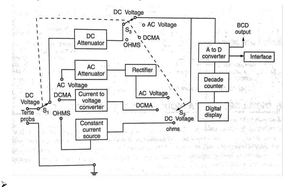
A commercial digital multimeter consist of several A to D converters, decade counters and display. It is basically dc voltmeter. In order to measure unknown current; current to
