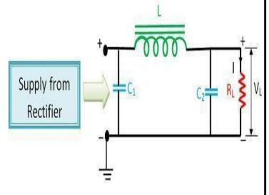
in series and another filter capacitor C<sub>2</sub> connected across the load. The shape of the circuit diagram of this filter circuit appears like Greek letter  $\pi$  (pi) and hence the name  $\pi$ -filter.
