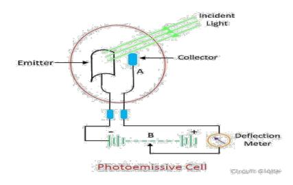
When the radiation of light fall on cathode plates the electrons starts flowing from anode to cathode. Both the anode and the cathode are sealed in a closed, opaque evacuated tube. When the radiation of light falls on the sealed tube, the electrons starts emitting from the cathode and moves towards the anode.
