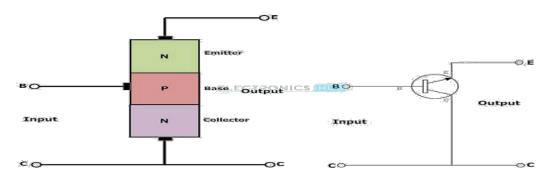
The ratio of change in emitter current ( $\Delta I_E$ ) to the change in base current ( $\Delta I_B$ ) is known ascurrent amplification factor in common collector (CC) arrangement i.e. $\gamma = \Delta I_E / \Delta I_B$
