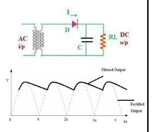
It is also called Capacitor Filter. It offers low reactance to ac &a very high reactance to the dc component. The capacitive reactance is  $X_C=1/2\pi fc$ , ford.c,
