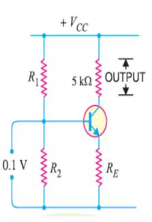
Due to transistor action, a much larger ( $\beta$  times the base current) a.c. current flows through the load R<sub>c</sub> in the output circuit. Since the value of load resistance R<sub>c</sub> is very high, a large voltage will drop across it.
